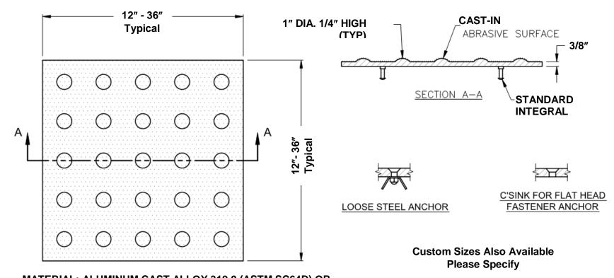
MATERIAL: ALUMINUM CAST ALLOY 319.0 (ASTM SC64D) OR MAG BRONZE CAST ALLOY ASTM B584.
